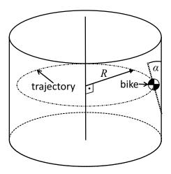
The bike and the rider are inclined at an angle  $\alpha$  to the wall. The angles  $\alpha$  that the bike can make with respect to the walls of the cage are limited by its handle bars to a certain minimum  $\alpha_{min} > 0$ . The types of the bike have a very high co-efficient of friction with the cage so that the types can only roll but not slip along the cage.
