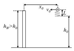
The above figure depicts a ball of mass m which is equipped on its lower side with a massless spring of uncompressed length  $L_0$  and spring constant k. The spring is initially compressed to a length  $L < L_0$ , as shown in the figure.
